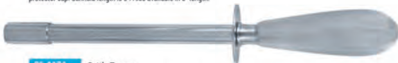
01-1174 Cattle Trocar This cattle trocar is used to relieve bloating. Complete with cannula, a hollow tube which remains when trocar is withdrawn to allow gas to escape. Stainless point. Metal handle 9.5" L. Tube is 5-1/2" L. 3/8" I.D.
